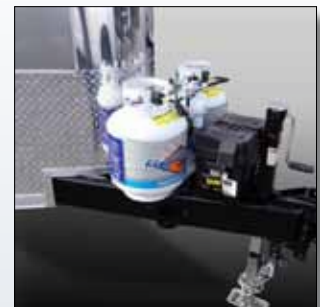
Dual 20# Propane Tank and Battery
